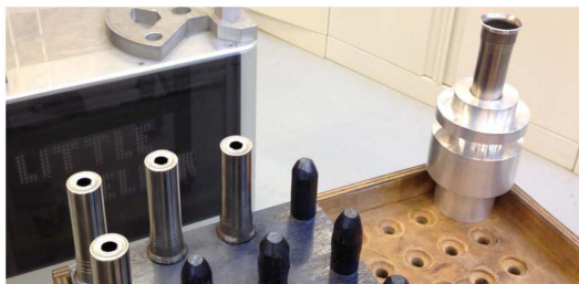
Fig. 8. Setup for task 2. One of the objects from the left fixture was to be placed up-side down into the fixture on the right.
